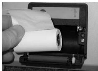
REMOVE EMPTY ROLL HOLDER PLACE NEW ROLL INTO THE MECHANISM, ENSURE THERMAL COATING IS UPPERMOST
