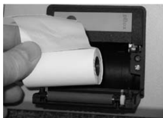
REMOVE EMPTY ROLL HOLDER PLACE NEW ROLL INTO THE MECHANISM, ENSURE THERMAL COATING IS UPPERMOST
