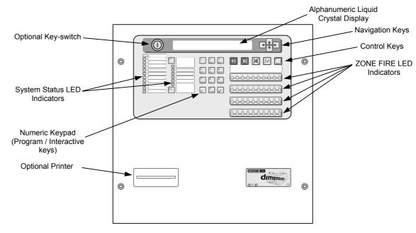
Figure 1 – Typical Controls and Indications
