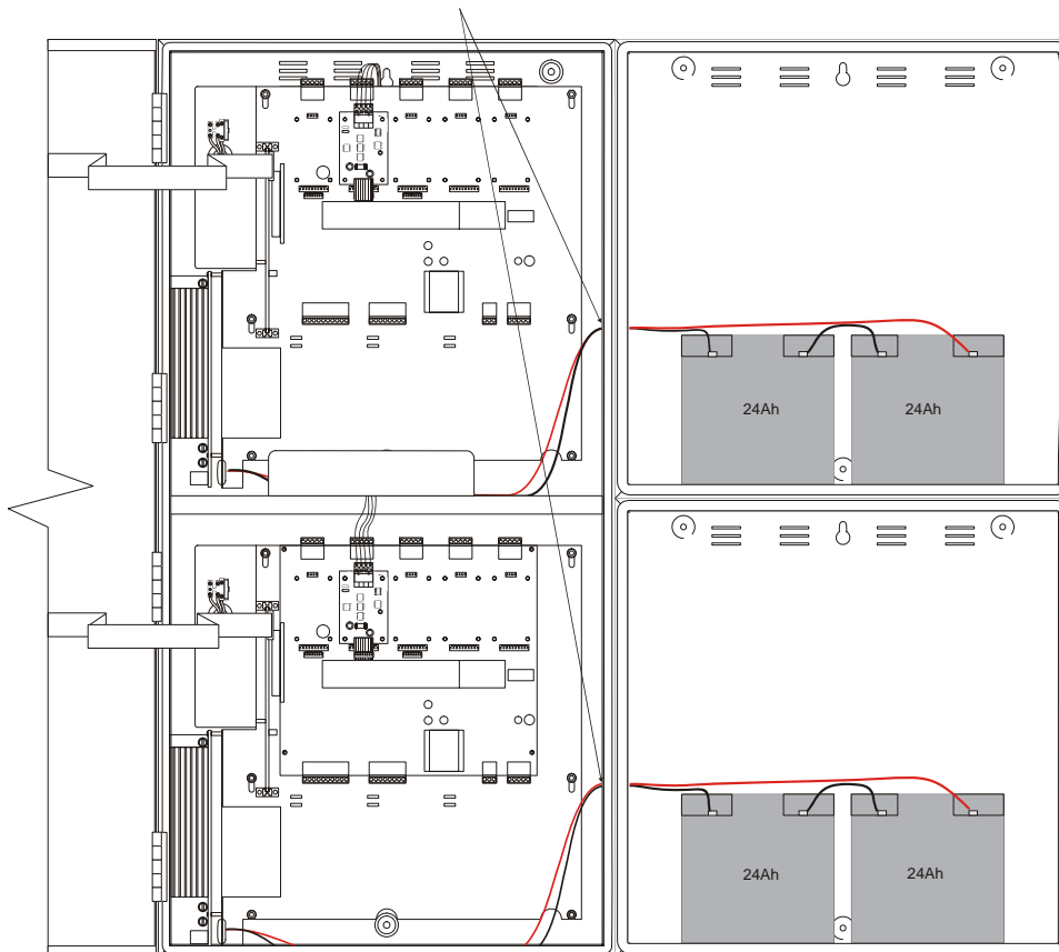
Figure 36 – ZX10Se Battery Installation – 17Ah or Greater
